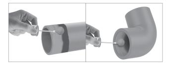
**Step 2:** fit all at once the ends to be welded, while the adhesive is wet, rotating 1/4 turn and keep the joint under manual pressure for approximately 30 seconds, till the adhesive is resistant.
