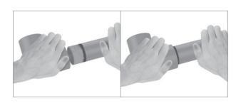
For 2 ½", 3" and 4", an additional procedure is necessary at the adhesive application step: apply a thicker layer of adhesive to the pipe extremity and after that apply an adhesive layer to the connection pocket;
